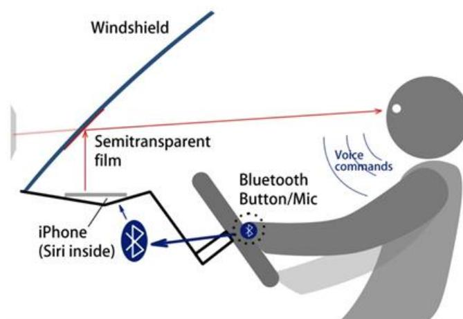
Figure 4: A human-vehicle interaction design aims to balance driver's hand, eye, ear and cognition resources.
