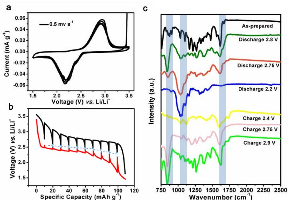
**Fig 2.** a, CV curves; b, galvanostatic intermittent titration technique (GITT) curves;
