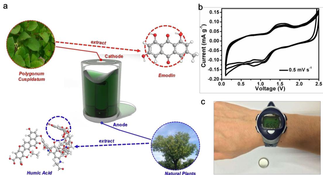
**Fig1.** a, Configuration of renewable-biomolecule-based full lithium-ion batteries with Emodin-based cathodes and Humic Acid-based anodes. b, CV curves of renewable-biomolecule-based full lithium-ion batteries. c, A coin-type full battery used to power an electronic watch.
